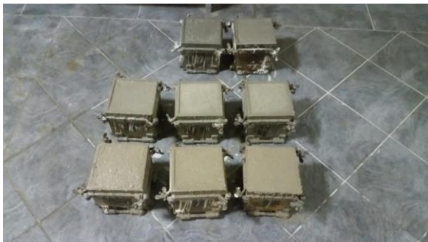
Figure 5: Prepared concrete samples
