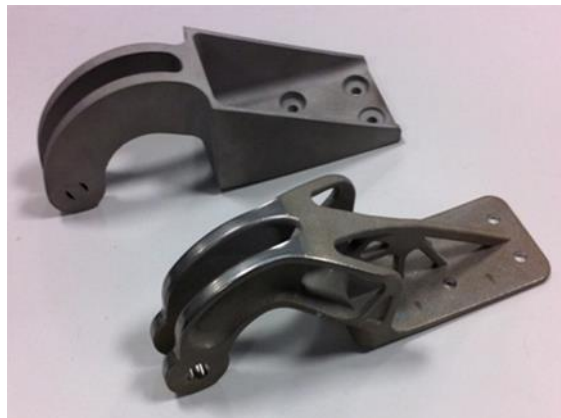
Figure 3: Product made by RP manufacturing technology [3]
