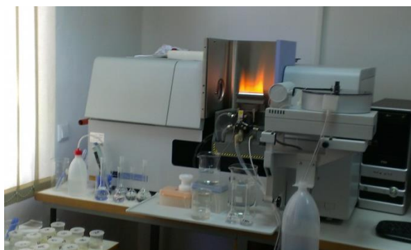
Figure 2: Atomic Absorption Spectrophotometer (Perkin Elmer)
