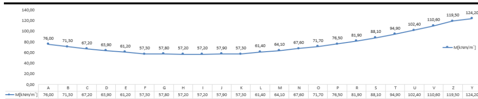
Graph 4: Bending moment in relation to the centre of gravity of the cross section of the foundation joint – sections A-Y
