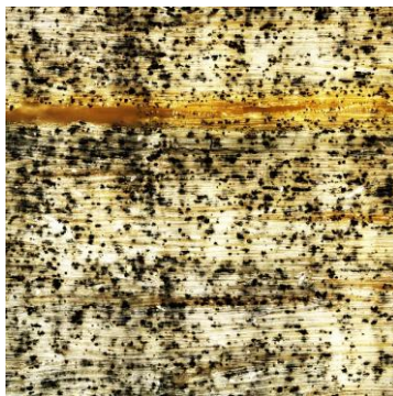
Figure 2: Development of the blue stain fungi on the surface of Norway spruce wood after 12 weeks of exposure as determined by Laser Scanning Confocal Microscopy.
