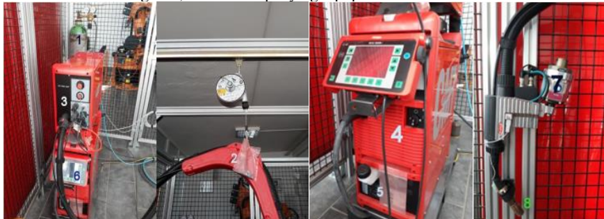
Figure 5: Welding unit FRONIUS CMT VR 7000 (with accompanying equipment)
