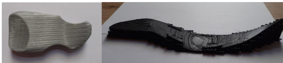
Figure 7: 3D printed chest and torso protectors
