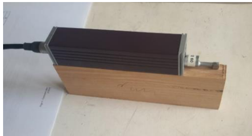
Figure 6: measuring the surface roughness with the MITUTOYO SURFTTEST SJ-201
