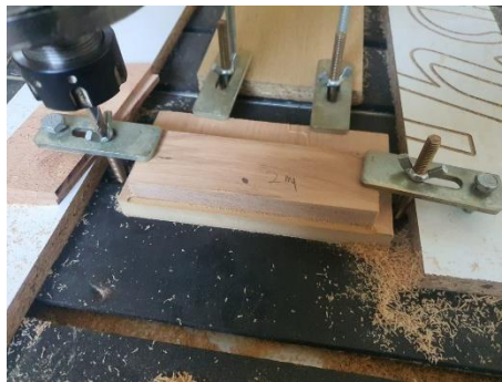
Figure 4: Specimen being routed on the cnc machine
