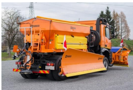
Figure 4: Truck with equipment for preventive sprinkling
