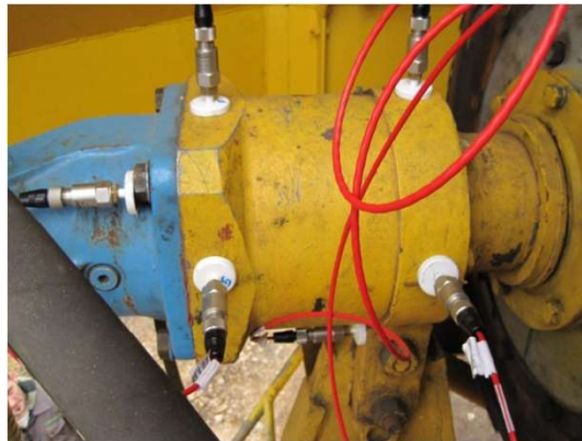
Figure 7. Sensor positions on UT reducers.
