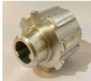
Figure 5. Machined notched element on a universal lathe machine.
