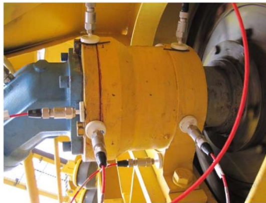
Figure 8. Positions of sensors on reducers IT.
