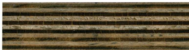
Figure 7. Cross-section of plywood overlaid with fiberglass prepreg after 192 days immersion in water
