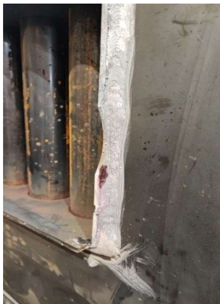
Figure 14. Detection of penetrant indications
